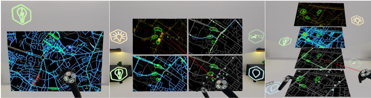
Figure 1: Left: Temporal multiplexing (*blitting*); center and right: spatial multiplexing — in a *grid* (center), and in our proposed *stack* (right). Shown as implemented for the user study, with controller interaction.
