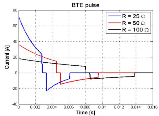
Figure 5: BTE waveform in function of the impedance.
