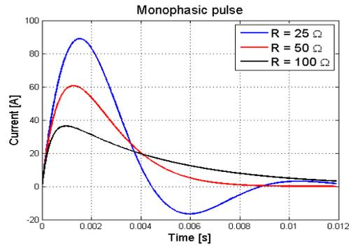
Figure 2: Lown waveform in function of the impedance.
