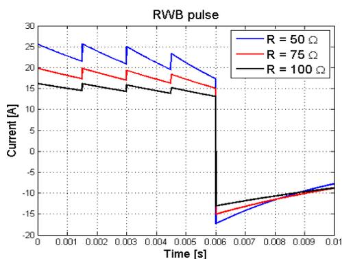
Figure 8: RBW waveform in function of the impedance.
