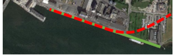
Figure 10: An illustration of a problem with the position estimation when panning to the right. The dotted red line is the position given by the estimator and the green line is the actual position of the waterfront.
