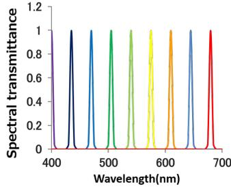
Figure 6: Examples of spectral transmittance of narrow bandpass filters equipped on a multiband projector.
