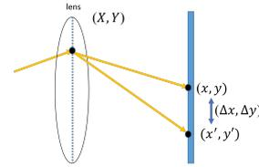
Figure 4: Optical aberration by lens distortion.
