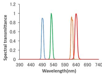
Figure 9: Spectral distribution of each projectors.
