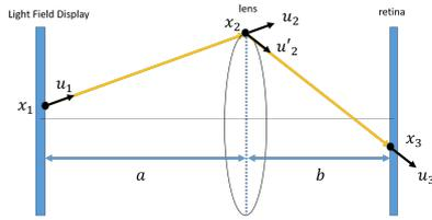
Figure 3: Ray tracing from light field display to observer.
