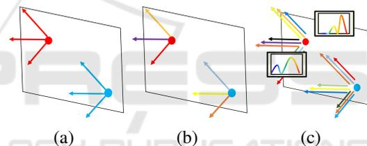
Figure 1: Difference between (a) standard displays, (b) light-field displays and (c) 5D light-field displays.
