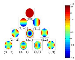
Figure 2: Zernike bases: numbers below each images indicates  $n$  and  $m$ .
