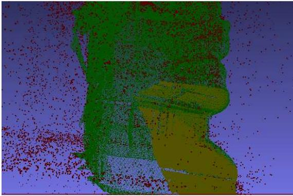
Figure 7: Point cloud density comparison. Red is Photogrammetry, Green is Low-cost scanner, and Yellow is Structured light scanner.
