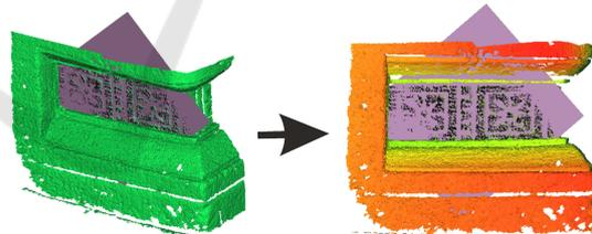
Figure 6: Left image: Mesh with with basis plane (rectangle) from RANSAC shape detector, Right image: Aligned mesh.
