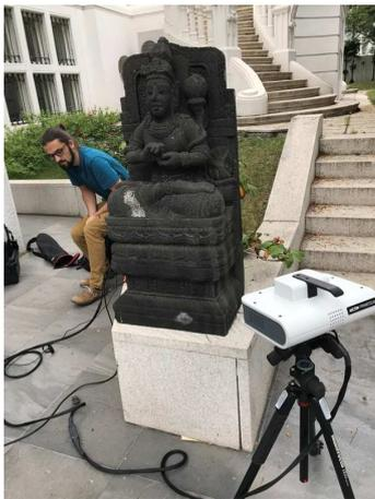
Figure 2: The outdoor scanning process of Structured Light Scanner to capture the sculpture.
