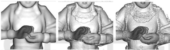
Figure 8: Direct view comparison of three different mesh. Left: low-cost scanner, middle: photogrammetry, right: structured light.
