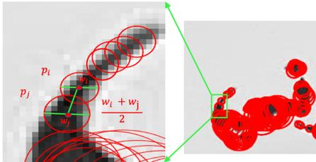
Figure 5: The grouping rule of two keypoints.
