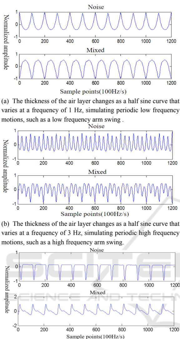
(a) The thickness of the air layer changes as a half sine curve that varies at a frequency of 1 Hz, simulating periodic low frequency motions, such as a low frequency arm swing .
