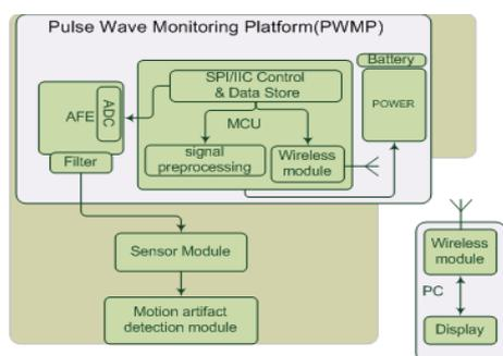
Figure 2: Block diagram of the Embedded system.
