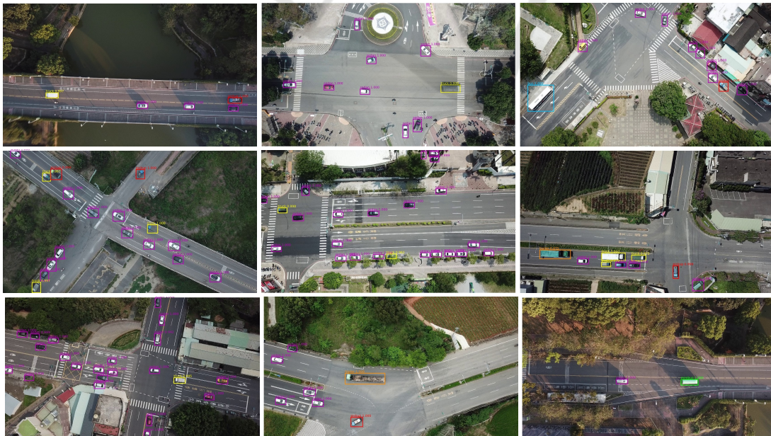
Figure 7: The results from our dataset and the modified Faster R-CNN with ReLU.
