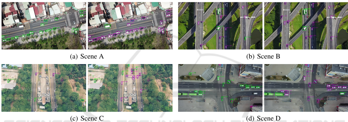
Figure 6: The results of Scenes A – D using the proposed vehicle detection approach. Left: Training with the VEDAI dataset. Right: Training with our VAID dataset.
