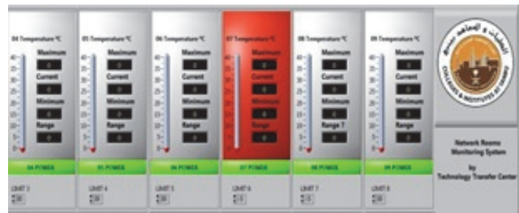
Figure 14: Sensors and power information displayed on main screen on the control room.
