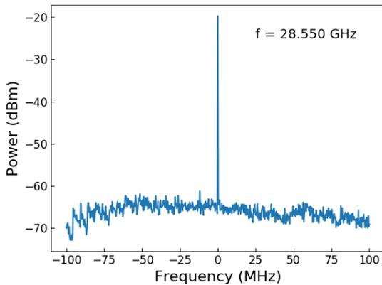
Figure 4: Beat note of the frequency comb repetition-rate.
