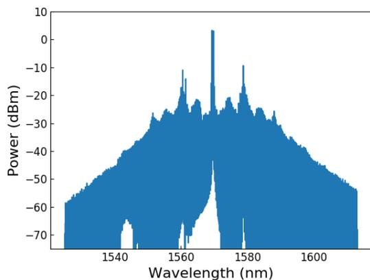
Figure 8: Frequency comb spectrum at  $f = 28.77$  GHz.
