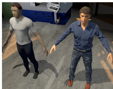
Figure 2: Full-body manikins – on the left the lowpoly version and on the right the highpoly version.
