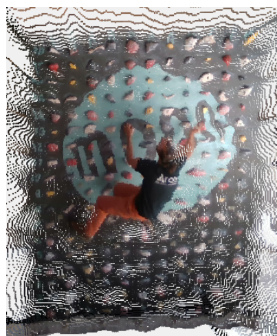
Figure 1: 3-D point cloud of a climbing scene captured by an Intel RealSense D435 RGB-D camera.
