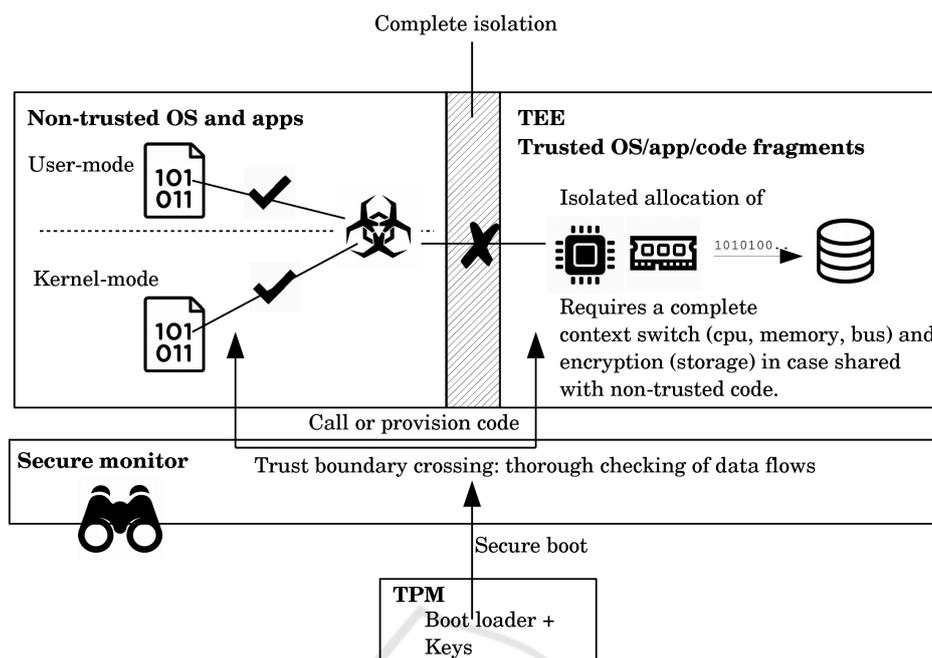
Figure 1: Components of a trusted execution environment (TEE).
