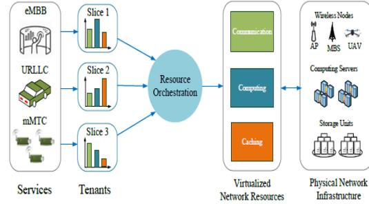
Figure 5: 1 Slicing in next-generation wireless networks (NGWNs) (Alcardo Alex Barakabitze, et al., 2019).
