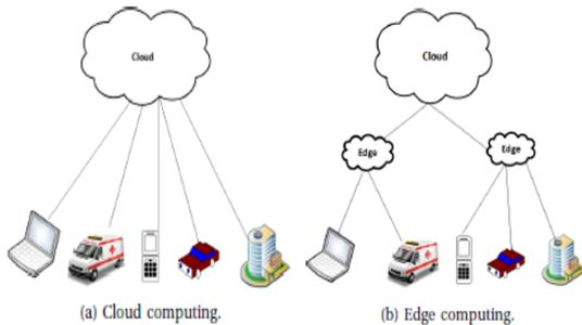
Figure 4: Present cloud computing (a) without edge. (b) with edge.
