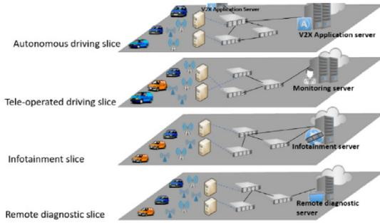
Figure 3: General architecture of network slicing.
