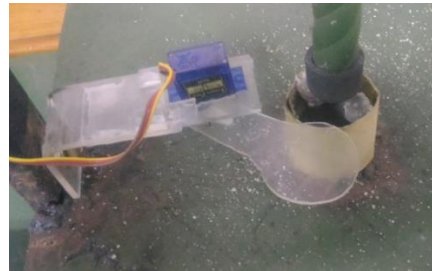
Figure 11: Servo Motor at condition 90°.
