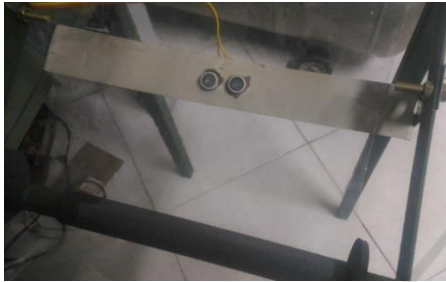
Figure 9: Position of the Ultrasonic sensor.
