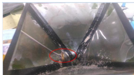
Figure 8: LDR Sensor Position in food container.
