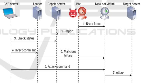
Figure 2: Steps and agents involved on Mirai attack (Koliass et al., 2017).
