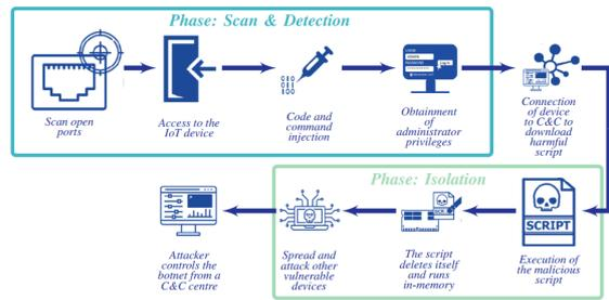
Figure 1: Botnet life cycle (Dietz et al., 2018).
