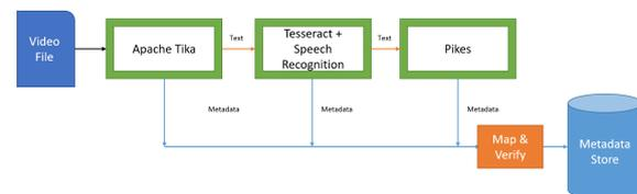
Figure 4: Video File Extraction Pipeline.
