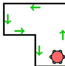
Figure 3: Top-Down illustration of a wall following robot traversing a room similarly to the robot that collected the ultrasound data. This robot has only 6 ultrasound sensors, as indicated by the blue circles. The green arrows show the path that the robot will take.
