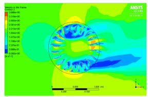
Figure 5 Contour Velocity 18 Blades 45° Blades Angle
