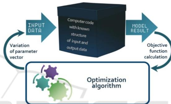
Figure 3: Scheme of the interaction between black box model and optimization algorithm.
