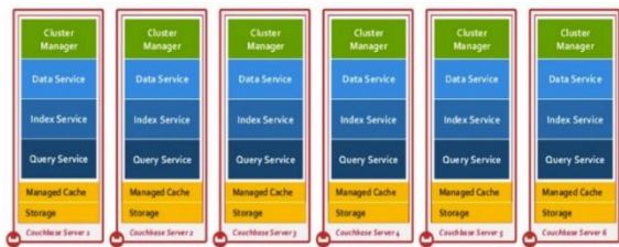
Figure 2: Couchbase Server architecture (“Couchbase Server architecture,” 2018).
