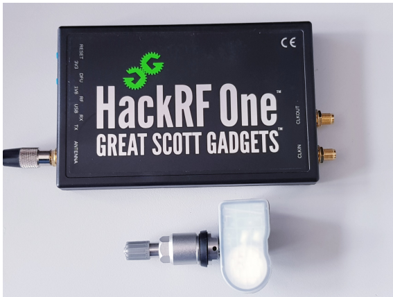
Figure 4: Analysis tools: HackRF and a commercial tire sensor.
