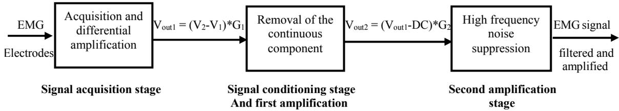
Figure 1: Different stages of the muscular signal extraction.
