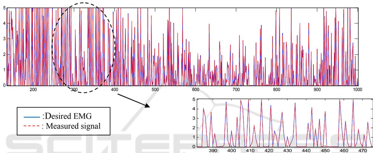
Figure 4: Simulation results of the desired EMG signal and the measured signal during the flexion movement of the elbow in position.
