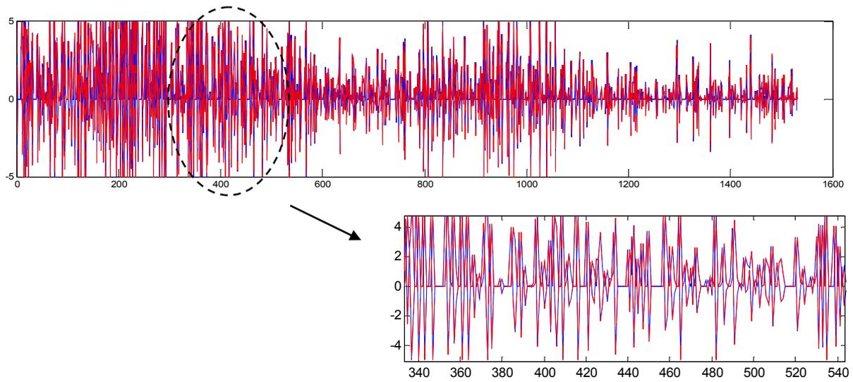
Figure 6: Simulation results of the desired EMG signal and the measured signal during the flexion movement of the elbow in velocity.
