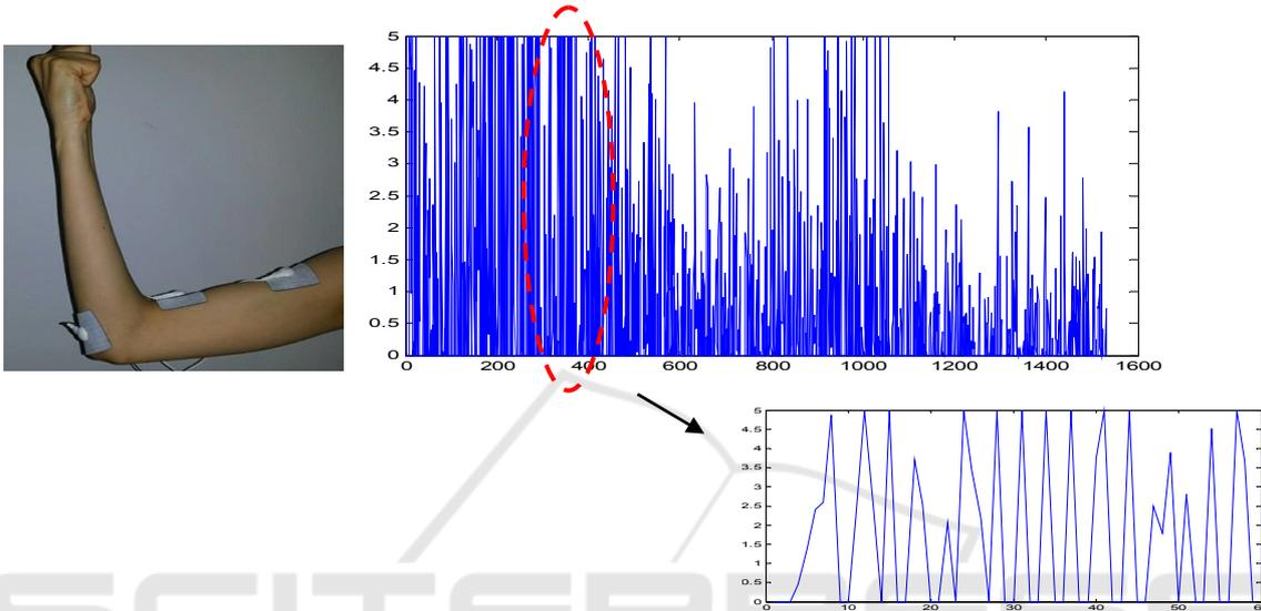
Figure 2: EMG signal obtained for a contraction movement of the elbow.
