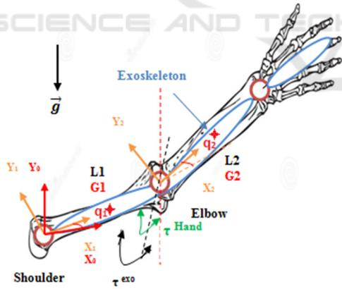
Figure 3: General configuration of a 2 DoF exoskeleton.
