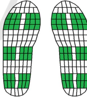
Figure 4: The sensors in the marked area were selected for plantar pressure measurement comparison with that of the Smart Socks System.
