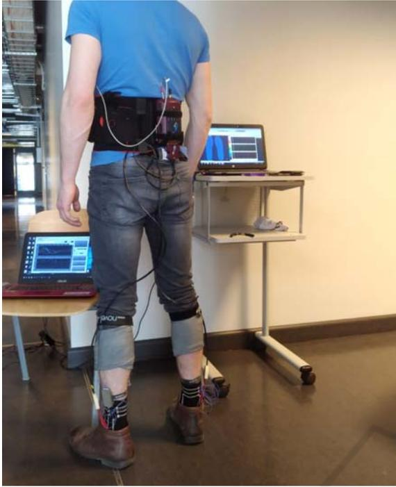
Figure 3: Test participant with the Pedar and the DPSS attached.
