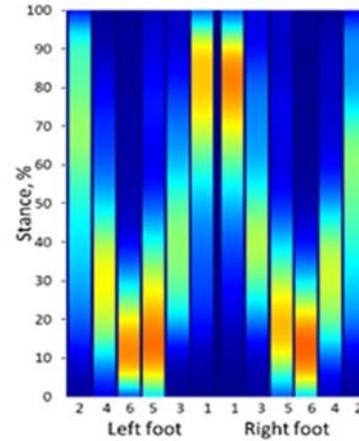
Figure 8: Example of a Pressure Wave diagram. The sensor measurement during the stance phase is represented as a color-bar plot with the colors representing the sensor measurement amplitude at each moment. The sensor numbering is according to that given in Fig. 2.
