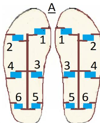
Figure 2: Sensor distribution and numbering on the Smart Socks system.
