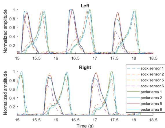
Figure 5: Example of normalized measurement for both systems, the sensor numbers for the DPSS sensors are according to Fig. 2 while the Pedar areas for each textile sensor are given in the Fig. 4.
