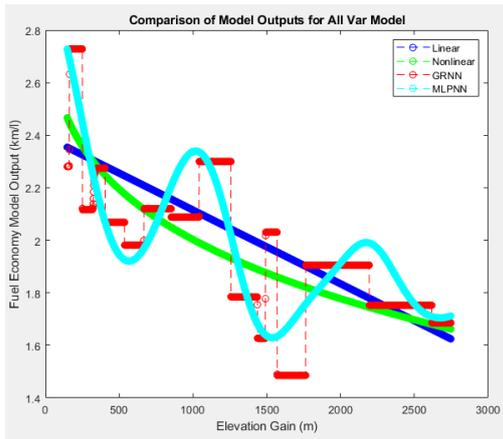
Figure 9: Elevation Gain vs Fuel Economy for all four model types, using low levels of regularization for neural models.
