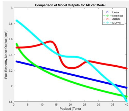
Figure 11: Payload vs Fuel Economy for all four model types, using low levels of regularization for neural models.
