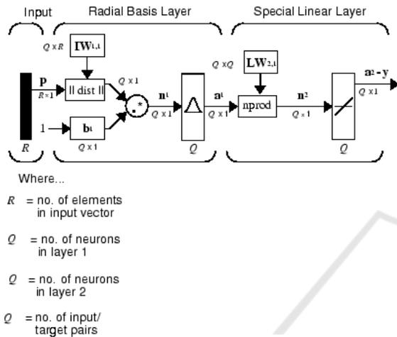
Figure 6: Architecture of the GRNN network.
