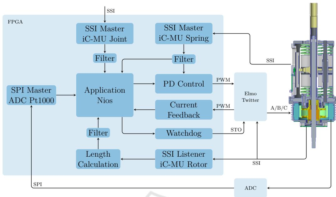
Figure 3: IP Cores acting as coprocessors on the application side of the FPGA system.
