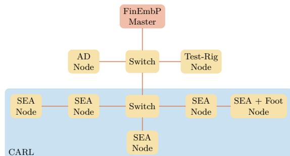
Figure 5: Topology of the FinEmbP network used during the experiment.
