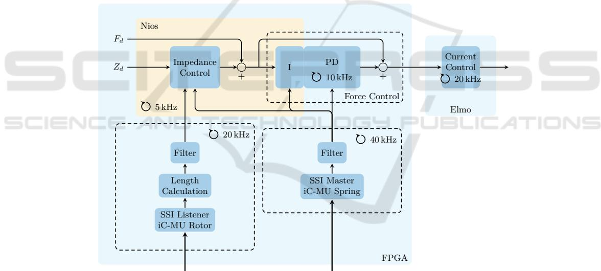
Figure 4: Distribution of the closed-loop cascades within the HW/SW system with the respective sampling frequencies.
