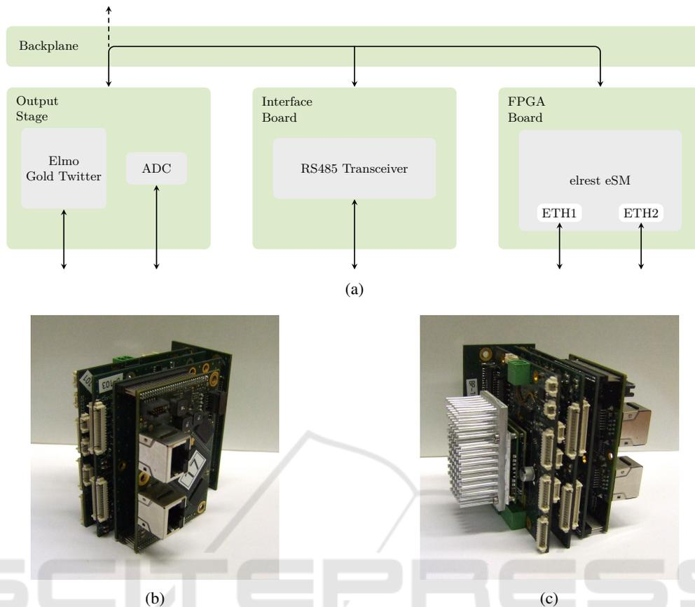
Figure 2: Embedded electronics developed for CARL– (a) the underlying modular concept and the implementation of (b) the FPGA module and (c) the Elmo based output stage. All the three boards are mounted on the backplane board.
