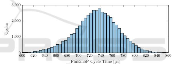
Figure 6: Histogram of the FinEmbP timing. The data is recorded with a network of seven nodes and the high-level walking control of CARL running on the master PC.
