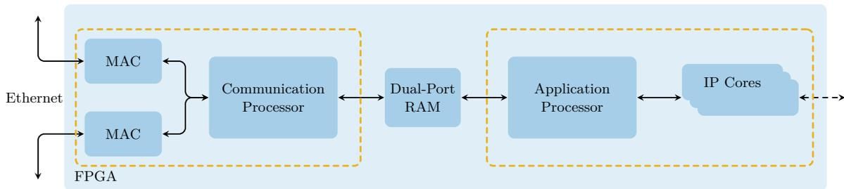
Figure 1: Task decomposition within the FPGA system. Adapted from (Schütz et al., 2014).
