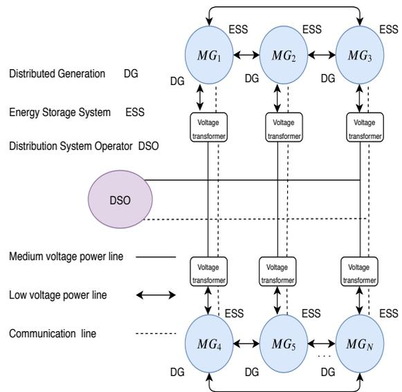
Figure 1: Networked MGs system architecture.
