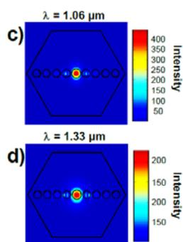
Figure 4: (a) Calculated effective refractive index of modes which can propagate in the fiber core when  $D_{core}$  was 3.0  $\mu\text{m}$ ,  $D_{rod}$  was 2.3  $\mu\text{m}$  and  $FF$  was 0.75. (b), (c) and (d) are intensity distribution of modes which correspond to red dots at 0.8, 1.06 and 1.33  $\mu\text{m}$ , respectively. (cont.)
