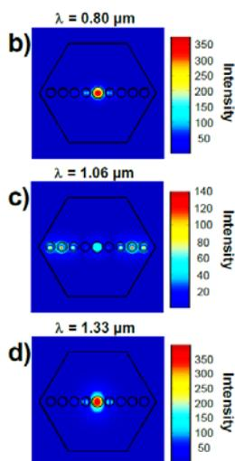
Figure 5: (a) Calculated effective refractive index of modes which can propagate in the fiber core when  $D_{core}$  was 2.5  $\mu\text{m}$ ,  $D_{rod}$  was 2.3  $\mu\text{m}$  and  $FF$  was 0.75. (b), (c) and (d) are intensity distribution of modes which correspond to red dots at 0.8, 1.06 and 1.33  $\mu\text{m}$ , respectively.
