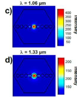
Figure 3: (a) Calculated effective refractive index of modes which can propagate in the fiber core when  $D_{core}$  was 3.0  $\mu$ m,  $D_{rod}$  was 2.5  $\mu$ m and  $FF$  was 0.75. (b), (c) and (d) are intensity distribution of modes which correspond to red dots at 0.8, 1.06 and 1.33  $\mu$ m, respectively.
