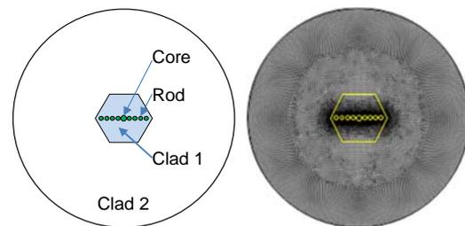
Figure 2: Schematic image of the fiber structure (left-side) and of the mesh distribution (right-side).
