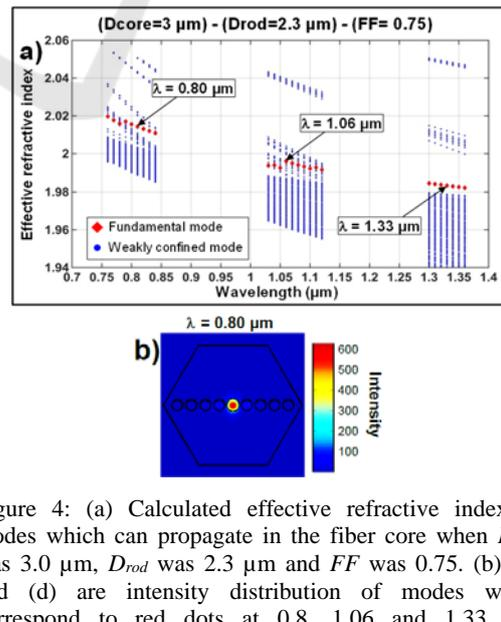
Figure 4: (a) Calculated effective refractive index of modes which can propagate in the fiber core when  $D_{core}$  was 3.0  $\mu$ m,  $D_{rod}$  was 2.3  $\mu$ m and  $FF$  was 0.75. (b), (c) and (d) are intensity distribution of modes which correspond to red dots at 0.8, 1.06 and 1.33  $\mu$ m, respectively.
