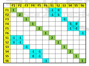
Figure 2: Schematic Laplacian Matrix generated from the bipartite graph in Fig. 1 – It has a diagonal Degree matrix (green background) and an Adjacency matrix (blue background) with minus signs by eq. (1). All matrix elements outside modules are zero-valued. (color online).
