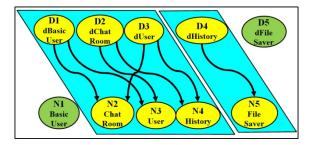
Figure 4: Chatroom Bipartite Graph - Arrows point from a "D" dependent vertex to an "N" non-dependent vertex. The bipartite graph itself already separates vertices into two "modules" (blue background). Isolated vertices (N1-BasicUser and D5-dFileSaver) are not connected at all to other vertices. (color online).
