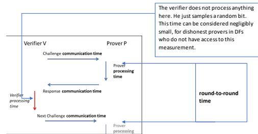
Figure 2: Communication & Computation Times in DB.
