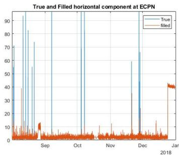
Figure 6: True and filled GPS displacement strength component at the ECPN station.
