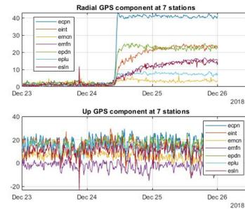
Figure 7: Horizontal displacement strength and up components at seven stations, immediately before and after the starting of the eruptive event occurred on December 24, 2018.
