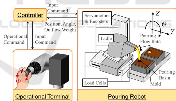
Figure 1: Tilting-ladle-type Pouring Robot.
