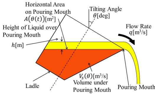
Figure 4: Cross Section of Pouring Process.
