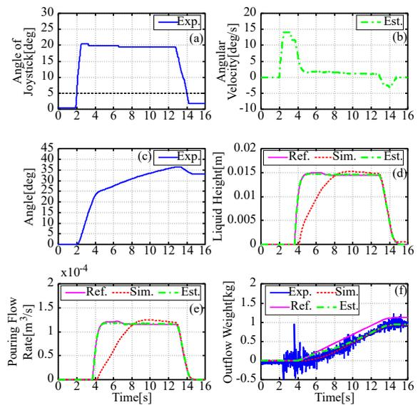
Figure 11: Experimental Results of Pouring Motion with Flow Rate Feedback Control and Flow Rate Feedback Control in Proposed Approach.
