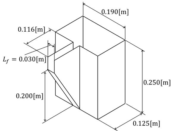
Figure 2: Geometry of Ladle.
