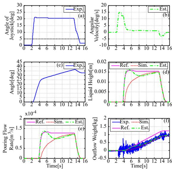
Figure 10: Experimental Results of Pouring Motion with only Flow Rate Feedforward Control in Previous Approach.
