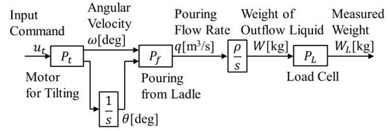
Figure 3: Block Diagram of Pouring Process in Pouring Robot.
