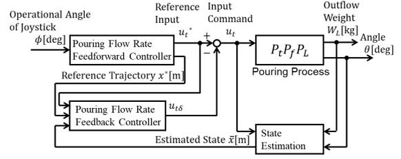
Figure 6: Block Diagram of Pouring Flow Rate Feedback Control in Operational Pouring Robot with Manipulatable Pouring Flow Rate.
