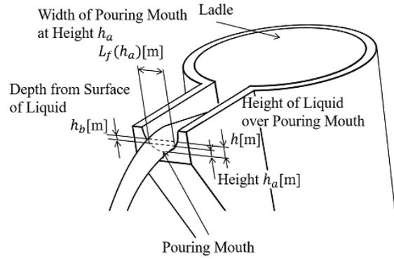
Figure 5: Parameters on Pouring Mouth.
