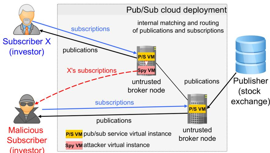
Figure 1: High-level overview of subscription leaks in a cloud deployed pub/sub service.
