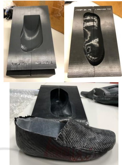
Figure 14: 3D printed male and female moulds, and prototype of carbon fibre cycling shoes.
