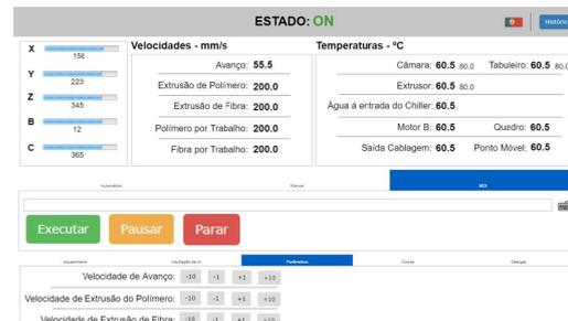
Figure 4: HMI - Fully Interactive Mockup.
