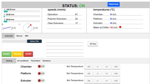
Figure 5: Home Screen of the Final HMI Design.
