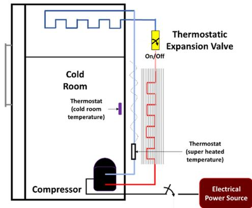
Figure 10: Conventional ON-OFF VCRC basic scheme.
