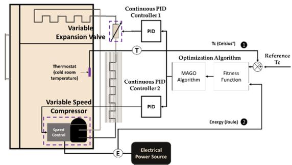
Figure 18: VCRC intervention with the third control strategy for temperature control and power source's energy reduction.
