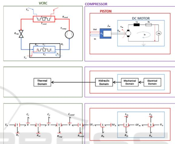
Figure 9: BG representation for the complete energy-based model of the VCRC.
