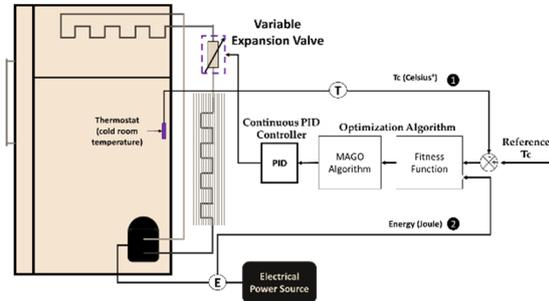
Figure 12: VCRC intervention applying the first control strategy for temperature control and power source's energy reduction.
