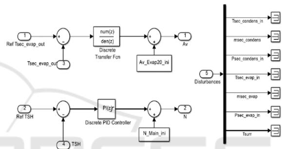
Figure 3: Discrete decentralized controllers included by default in the refrigeration control benchmarking (Bejarano *et al.*, 2018).
