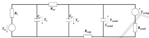
Figure 8: Base model of a VCRC. Adapted from (Schné, Jaskó and Simon, 2015).
