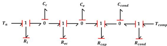
Figure 7: BG base model of a VCRC (thermal behaviour).
