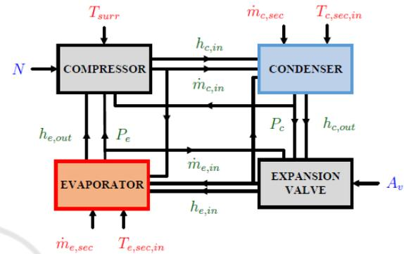
Figure 2: A vapour compression refrigeration cycle scheme (Bejarano, 2017).
