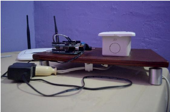
Figure 3: Stationary node of a domotic system - In this image you can see the stationary node of the domotic system. It includes an Arduino connected to the Wi-Fi Shield, a router for the wireless connection to the subnet, a power card with 4 relays and a socket for the connection of household appliances.
