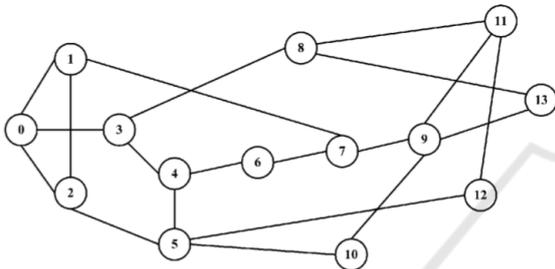
Figure 3: Transport backbone network, NSFnet.
