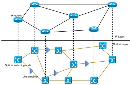
Figure 1: IP-Over-EON Architecture.
