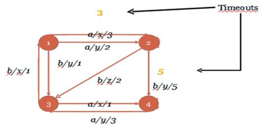
Figure 3: Finite state machine with timeouts.
