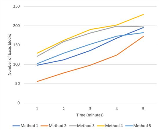
Figure 7: Shows the number of different basic blocks executed by each fuzzing method for *zlib* library. The horizontal axis shows the results for different moments of time (minutes).
