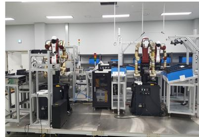
Figure 1: The developed robotic manufacturing system to pack cellular phones with multiple industrial dual-arm robots.
