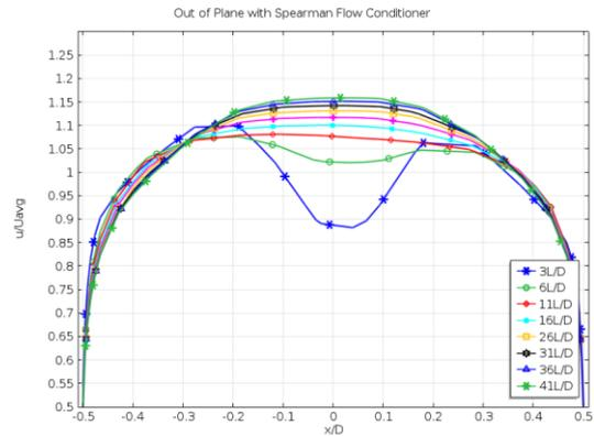
Figure 10: Velocity profiles downstream of NEL Spearman flow conditioner (double out of plane 90° elbows).
