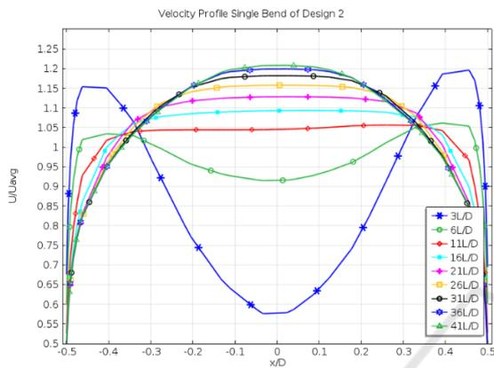
Figure 16: Design 2 velocity profile.
