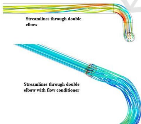
Figure 14: Velocity field US and DS of flow conditioners.
