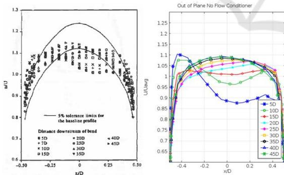
Figure 5: Velocity profile (double out of plane 90° elbows).
