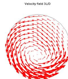
Figure 12: Velocity field through double out of plane 90° elbows (Re=1.5E6).
