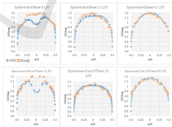
Figure 7: Velocity profile NEL Spearman: top: single 90° elbow, bottom: double out of plane 90° elbows.
