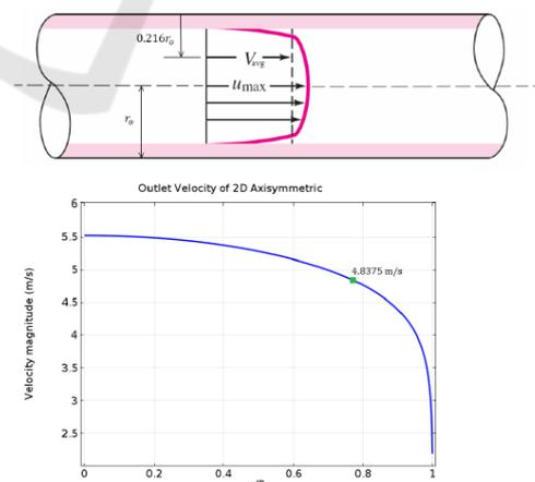
Figure 3: Velocity profile at outlet of 2D model ( $V_{avg}=4.8375$  m/s).
