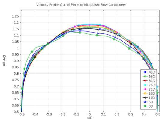
Figure 9: Velocity profiles downstream of Mitsubishi flow conditioner (double out of plane 90° elbows).
