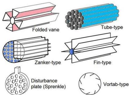
Figure 1: Different types of flow conditioners (Miller, 1996).
