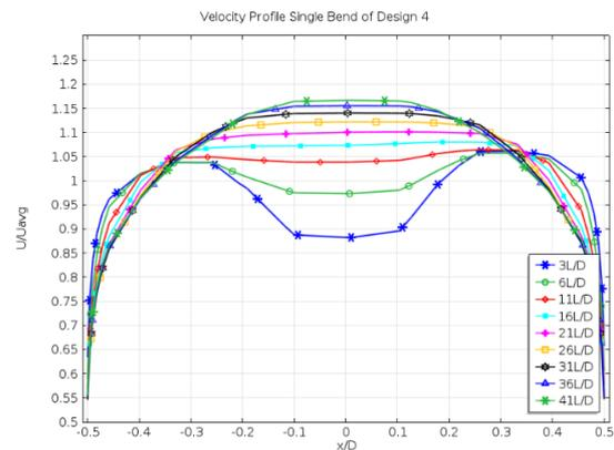
Figure 18: Design 4 velocity profile.
