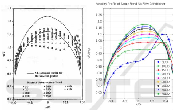
Figure 4: Velocity profile (single 90° elbow).
