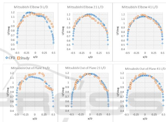
Figure 6: Velocity profile Mitsubishi: top: single 90° elbow, bottom: double out of plane 90° elbows.
