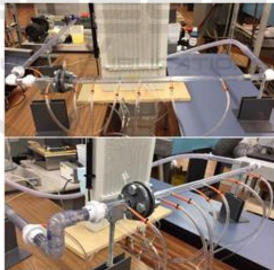
Figure 19: top: Flow loop with a single 90° elbow and bottom: double out of plane 90° elbows.
