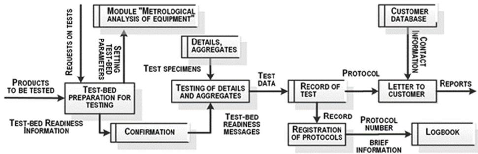
Figure 2: Diagram of data flows of the process “Testing of units and vehicle parts”.
