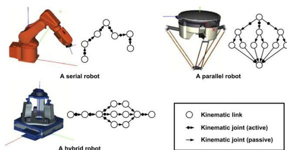
Figure 1: Industrial robot configurations. (Xiao et al., 2014).
