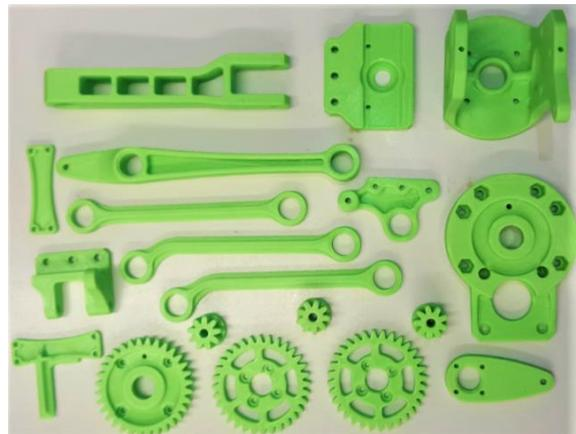
Figure 5: 3D printed components of RobotArm.
