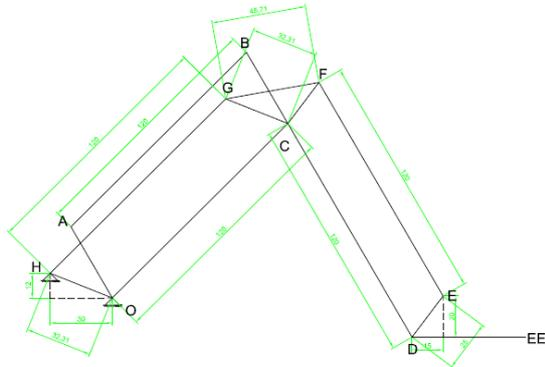
Figure 6: RobotArm dimensions.
