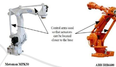
Figure 3: Different quasi-serial manipulators. (Shaik et al., 2012).
