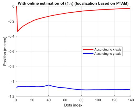
Figure 8: Estimates of  $\delta_x$  and  $\delta_y$  for the case "offset estimation and PTAM" ( $\gamma=10\text{deg}$ ).
