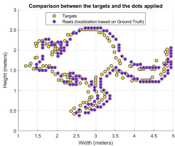
Figure 7: Desired and obtained drawings for the case "no offset estimation and GT" ( $\gamma=10\text{deg}$ ).
