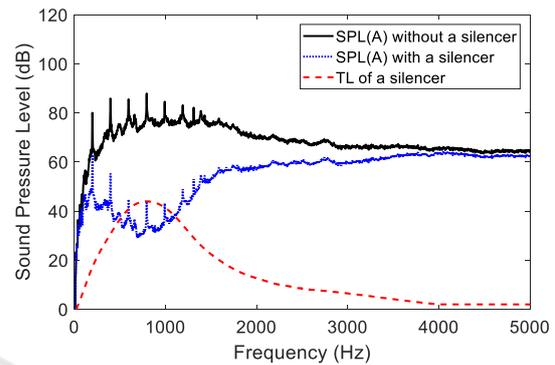
Figure 12: Reduced noise spectrum of the axial fan with the silencer, that is evaluated by subtracting TL from the measured noise spectrum of the axial fan, itself.
