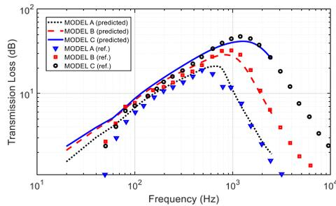
Figure 7: Comparison of the predicted TL of silencers (without a pod [model A], with a rigid pod [model B] and with an sound absorbing pod [model C], respectively) with results in the reference.
