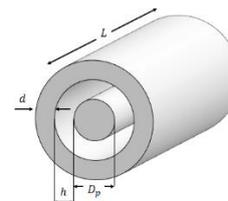
Figure 6: Silencer models for analysis verification.
