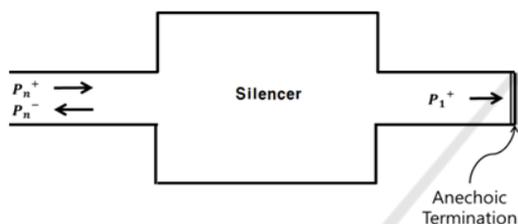
Figure 1: Layout for evaluation of transmission loss.
