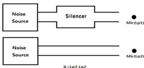
Figure 2: Layout for evaluation of insertion loss.
