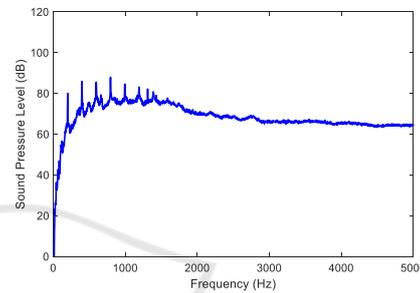
Figure 5: Measured noise spectrum of axial flow fan.
