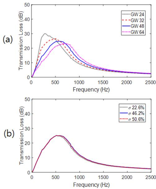
Figure 11: Influence of corresponding design variable change on TL of the silencer as (a) sound absorbing material density in unit of  $\text{kg}/\text{m}^3$  and (b) porosity of the perforated tubes.
