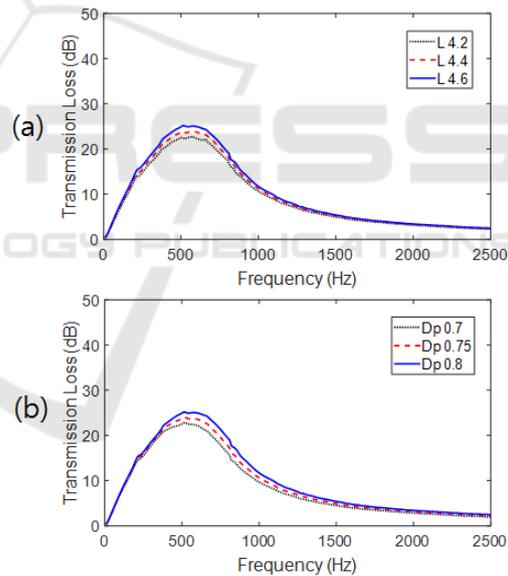
Figure 10: Influence of corresponding design variable change on TL of the silencer as (a) silencer length and (b) sound absorbing pod diameter.
