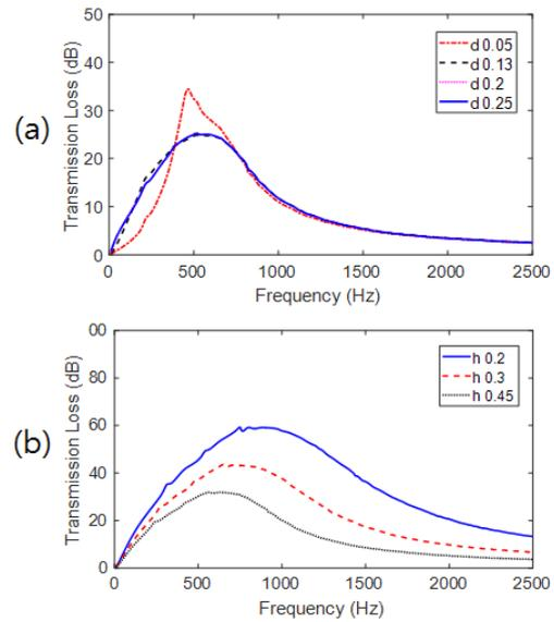
Figure 9: Influence of corresponding design variable change on TL of the silencer as (a) outer sound absorbing layer thickness, (b) air flow gap thickness.
