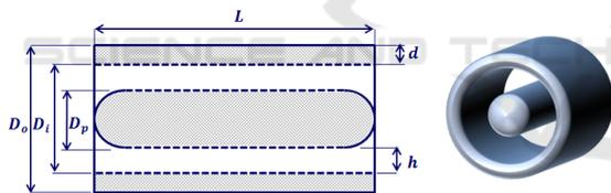
Figure 8: Design model of the circular-type pod silencer.
