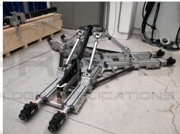
Figure 1: The Hexafloat : a 6DOF PKM.
