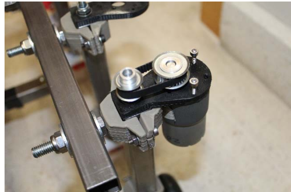
Figure 16: Details of the transmission between the electrical motor and the linear actuator. 30 MXL 025 and 22 MXL 025 timing pulley and 44 MXL timing belt.
