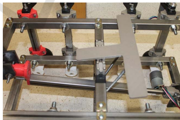
Figure 18: First built prototype (1:2 scale). Details of the ninth linear actuator and mechanism that guarantees the horizontal position of the users.
