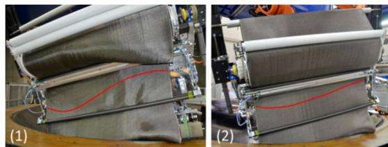
Figure 13: Material tension and fibre angle without buffer (1) and with buffer (2).
