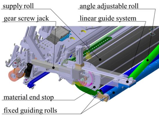
Figure 7: Material buffer in detail.
