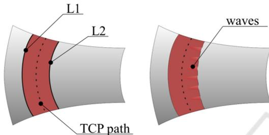
Figure 1: Generic sketch of a textile ply on an aircraft fuselage with the path of Tool Centre Point (TCP).
