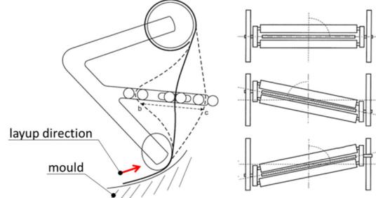
Figure 2: Material buffer concept.
