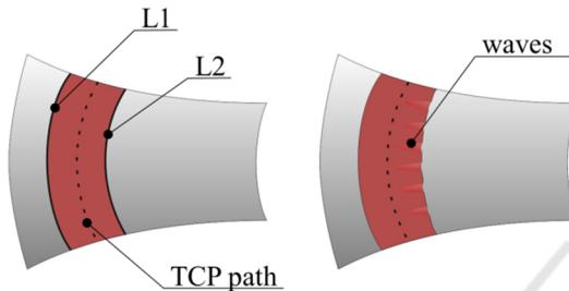
Figure 1: Generic sketch of a textile ply on an aircraft fuselage with the path of Tool Centre Point (TCP).
