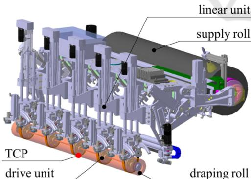
Figure 5: End effector without material buffer.
