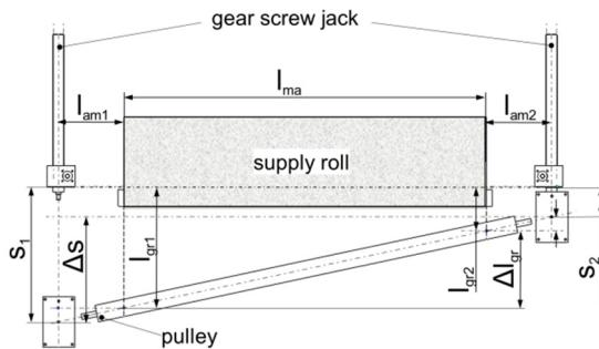
Figure 9: Geometric quantities for calculating the difference  $\Delta l_{gr}$  of the lengths  $l_{gr1}$  and  $l_{gr2}$ .
