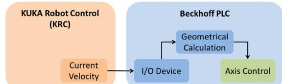
Figure 11: Schematic sketch of the control structure for the adaptable material buffer.
