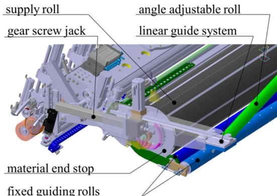
Figure 7: Material buffer in detail.
