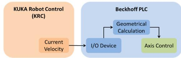
Figure 11: Schematic sketch of the control structure for the adaptable material buffer.
