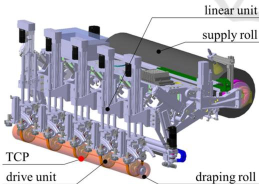
Figure 5: End effector without material buffer.
