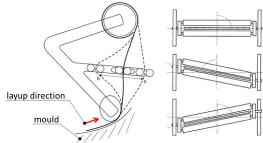
Figure 2: Material buffer concept.
