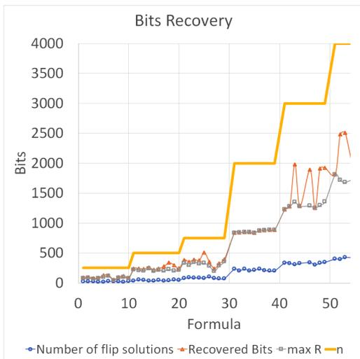
Figure 2: Total number of bits recovered by Flip Search and XORing process. The solid line denotes the number of bits (variables) in the original formula for each obfuscated one.
